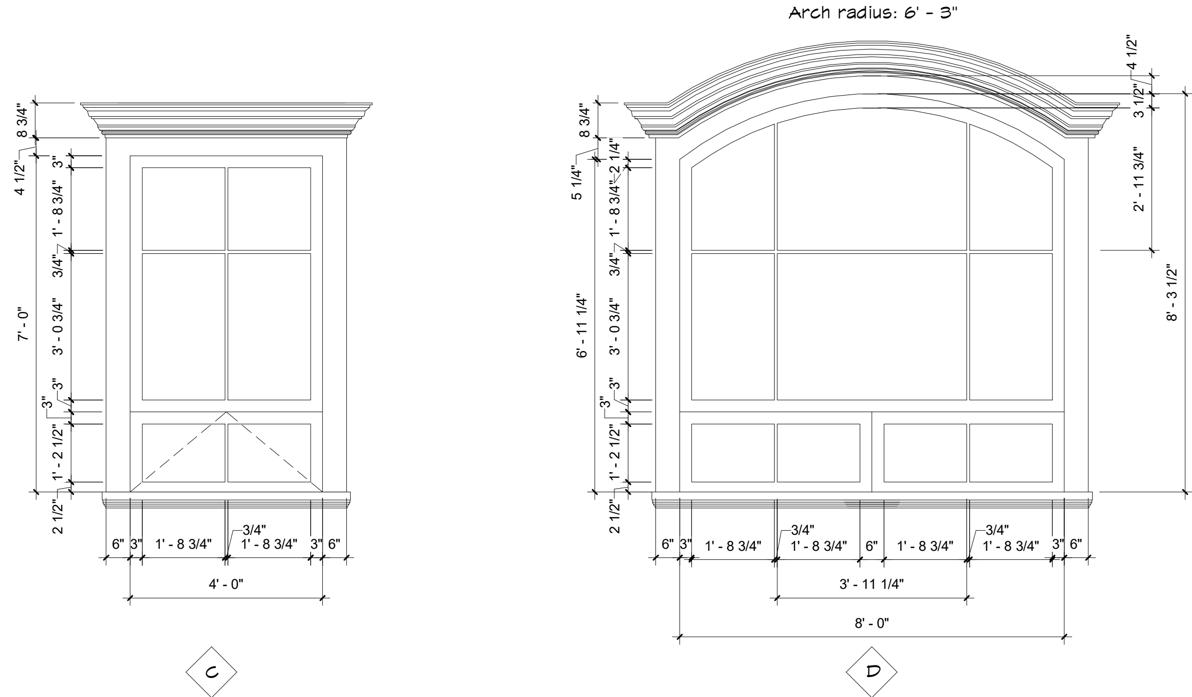
2 Window Head Elevation Detail 3" = 1'-0"
