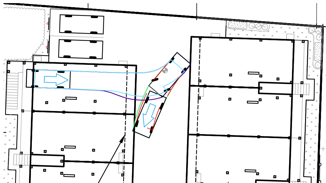
PROP. DRIVEWAY UNDER BUILDING OVERHANG (TYP.) PROP. BUILDING PILING FOUNDATION (TYP.) PASSENGER CAR BACKING UP FROM REAR UNIT (SCALE: 1"=20')
